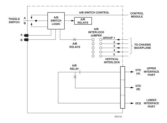
Figure 2-8. A/B Switching Module Simplified Circuit Diagram
